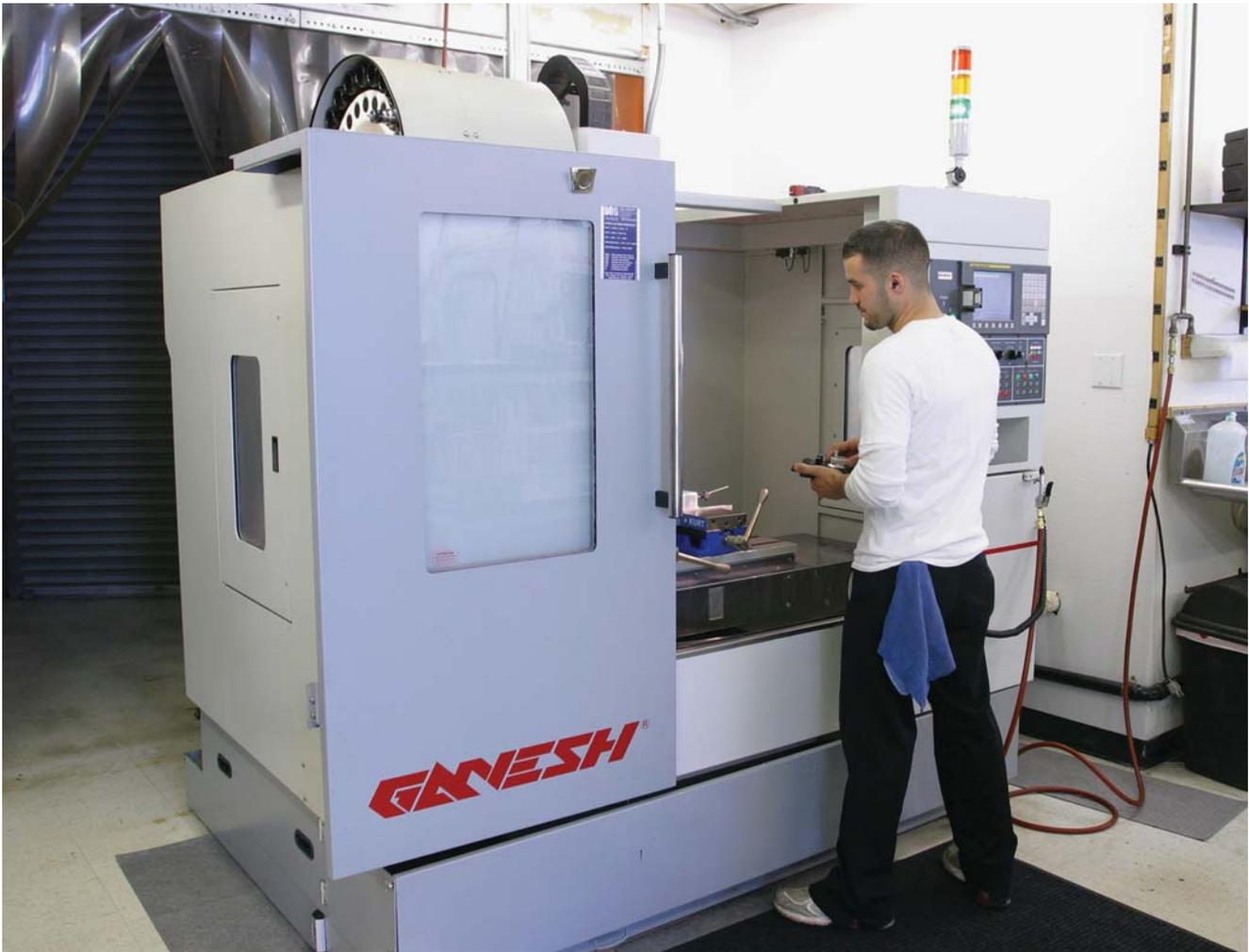
Roger de la Torre, CNC operator, sets up to run parts for Cisco Systems on PDM's new 4-axis Ganesh 2818 VMC. System work envelope is 70.8" x 80.9" x 99.6". Work cube is 9938.49 cubic inches. Spindle speed ranges from 60-8,000 rpm.
