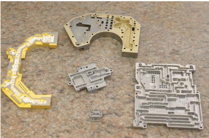
**Typical parts produced by Precision Dynamic Machine. On the left is an RF module made of gold-plated and ground Carpenter 49. The top part is an aluminum chassis, plated with nickel and alodine. The righthand part is made of Kovar for use in RF jamming. The middle part is missile component made of Carpenter 49. The small piece on the bottom is made of titanium for a commercial product.**
